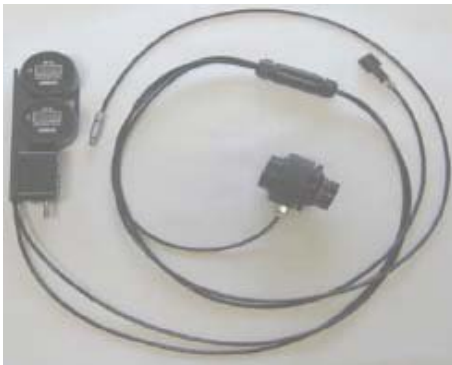
Multi Sensor Head with PPO2-meter, HUD and cable with Fisher connector
