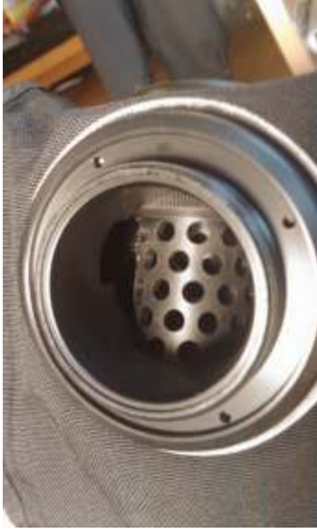
P-port cage threaded and secured to the p-port.
