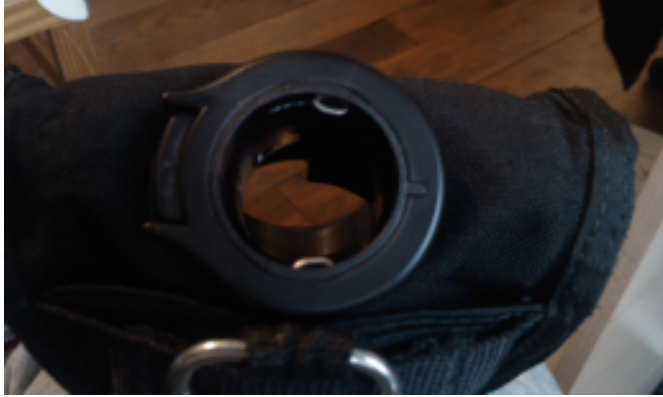
P-port with plug removed.
